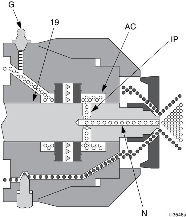
**3.** Remove grease fitting cap. Using grease gun (Y), dispense grease into fitting (G) until grease mist sprays from mix chamber nozzle (N). Do not over-grease; use 2 shots maximum. Do not spray grease mist on sprayed material.
